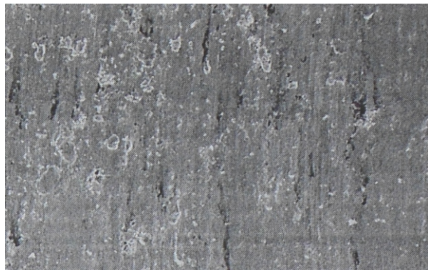
Fig. 5. Scanning electronic microscope image of the surface of drilling holes Al/15%SiC/4% Gr (speed 3000 rpm feed rate 0.05 mm/rev)
