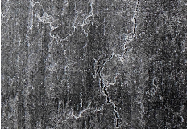
Fig. 6. Scanning electronic microscope image of the surface of drilling holes Al/15%SiC/4% Gr (speed
